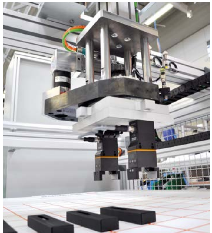
Pick & Place mittels 3-Achs-Portal
