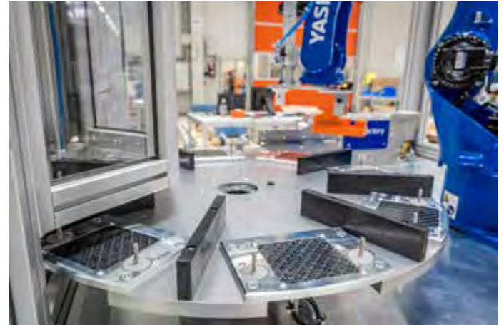
The workpieces for the hybrid welding are transported in the robot cell to a rotary indexing table.
