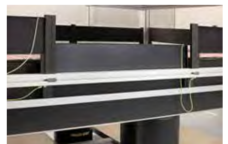
View of the laser protection plates.
