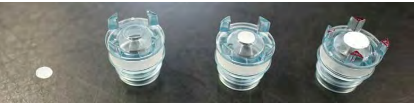
So simple and yet so demanding: The gauze is placed on the membrane cap, then the actual membrane.
