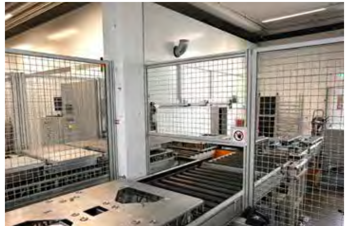
Heavy Metal: A MiniTec RMS conveyor system is used to transport the heavy-duty weigh cells.
