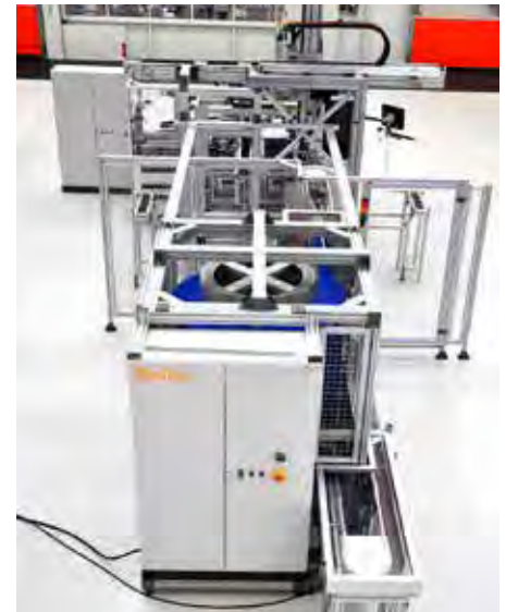
Thanks to the buffer capacity of the spiral conveyor, production machines can be loaded fully autonomously and the production thus automated further.
