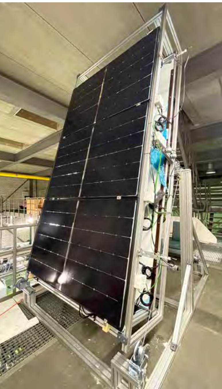
The Energy and Information Department of the HTW Berlin uses a test setup to determine the optimum back ventilation distance of PV modules.
